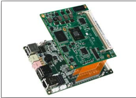
Figure 3. Computer-on-Module concept, compact baseboard and COM Express module
