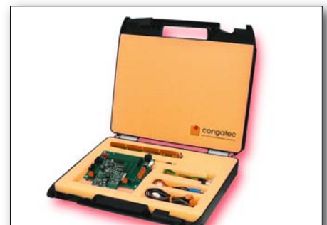
Figure 2. congatec Smart Battery Management Starter Kit for rapid evaluation
