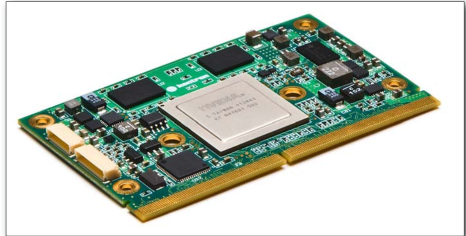
Figure 3. The ULP-COM-sAT30 measures just 82 x 50mm and is equipped with Nvidia Tegra 3 quad-core processor with 800 MHz.
