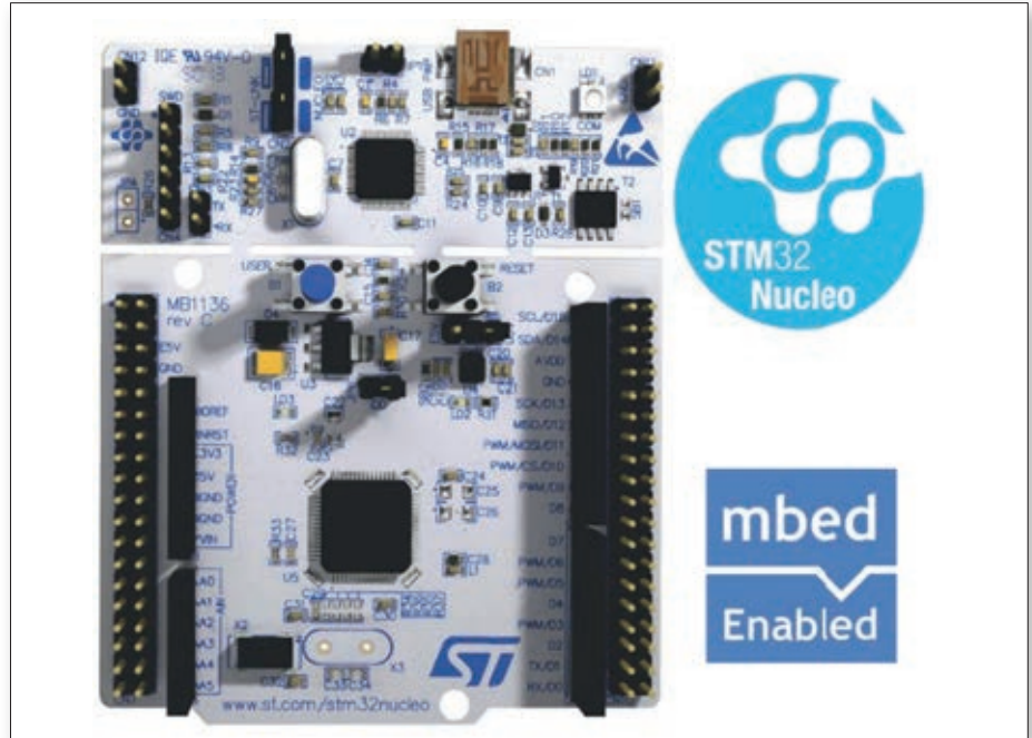
Figure 2. The OSHW Nucleo is about $10, includes free mbed.org software tools and is also supported by KEIL tools. STM32 Nucleo is compatible with most Arduino shields.
