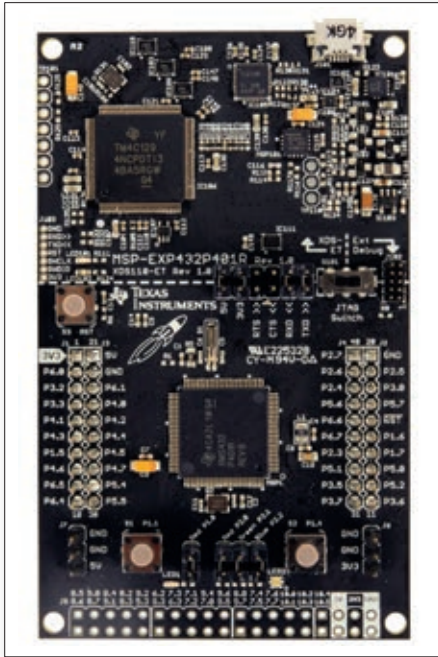
Figure 1. Latest Texas Instrument (OSHW) LaunchPad features the MSP432 processor and is aimed at the portables, wearables, smart grid, medical, and automation control markets.
