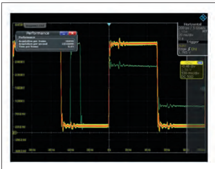
Figure 2. Rare signal faults are found quickly thanks to the high acquisition rate of one million waveforms per second.
