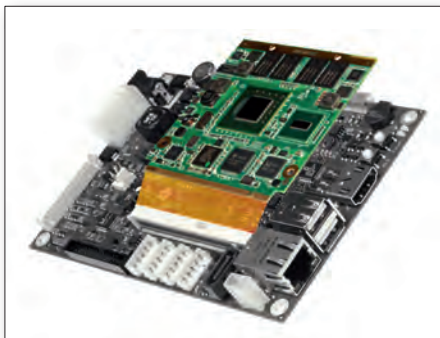
Figure 2. Qseven Computer-on-Module concept with carrier board and computer module
