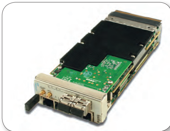
Figure 1. By providing a GPS receiver and IEEE1588/SyncE on a 40G MicroTCA Carrier Hub (MCH), today MicroTCA systems can provide precision timing for many applications.
