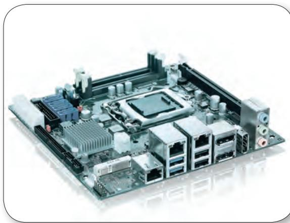
*Embedded motherboard mITX-KBL-S-C236 with a socketed 7th generation Intel Core processor*
