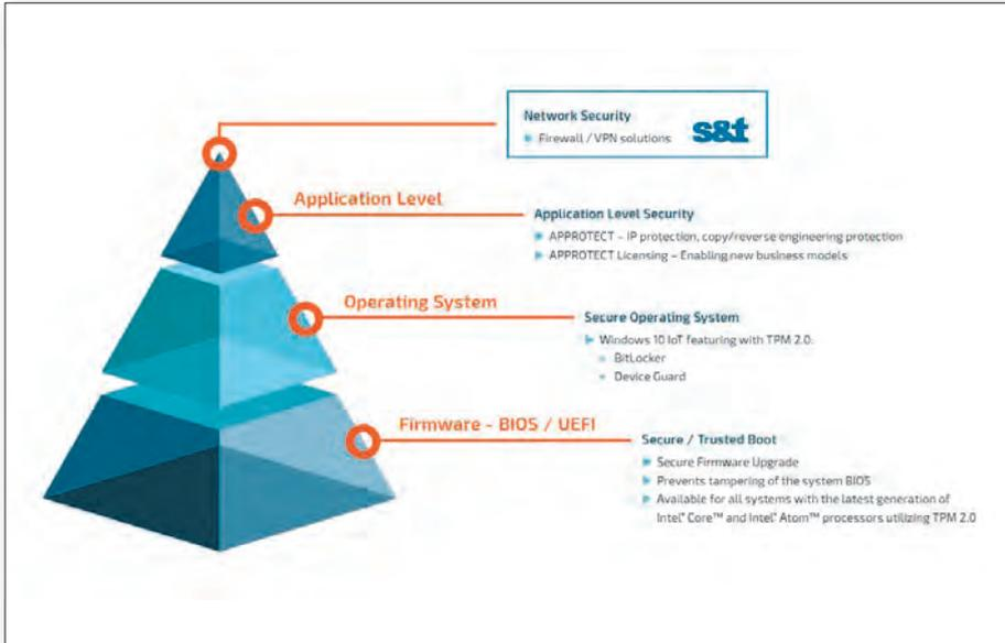
Kontron Security Pyramid: 3 levels of security from trusted boot to secure application execution.
