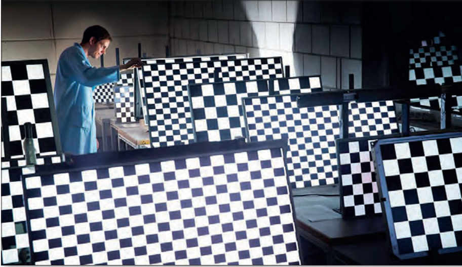
Figure 4. Stress test in the Data Modul climate chamber
