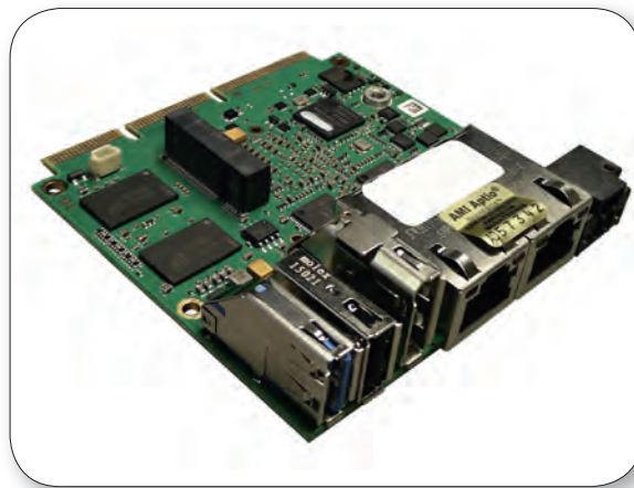
Figure 1. With the ADLE-3800SEC a Microsoft Azure certified 75 mm x 75 mm Edge Connect SBC with Intel E3800 ATOM processor is offered.
