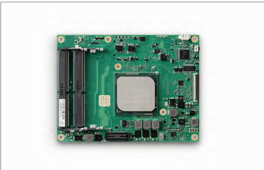
Figure 2. Thanks to their 10 GbE interfaces and massive PCIe support, the brand-new COM Express Type 7 Computer-on-Modules from ADLINK Technology are tailored for Industry 4.0 server and collaborative robotic applications
