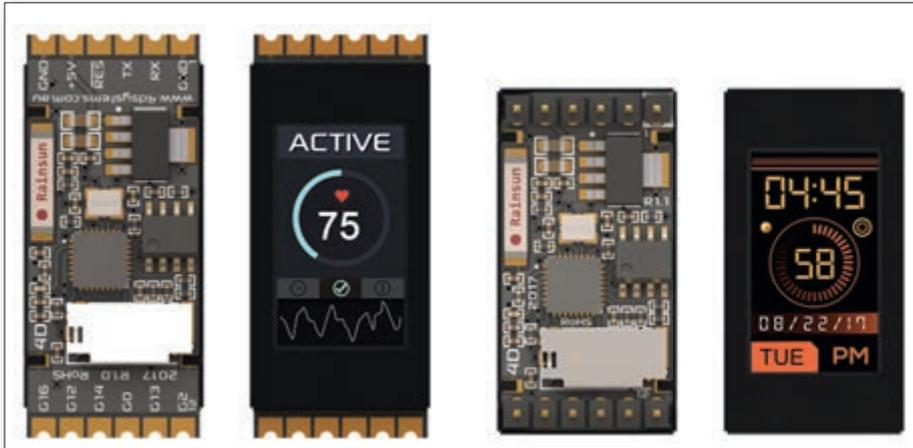
Figure 1. IOD-09 - images of surface-mount and through-hole versions
