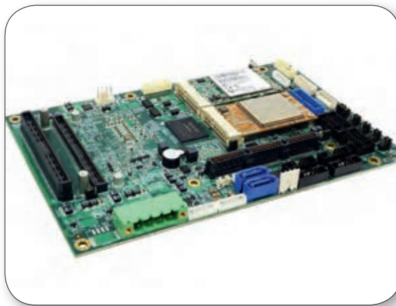
Figure 1. EBX form-factor with PCIe/104 Expansion connector and integrated MiniPCIe for I/O expansion
