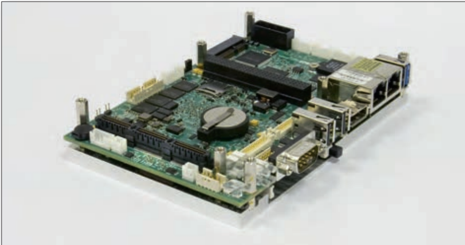
Figure 3. Industry form-factor 3.5" meets PCIe/104 expansion concept
