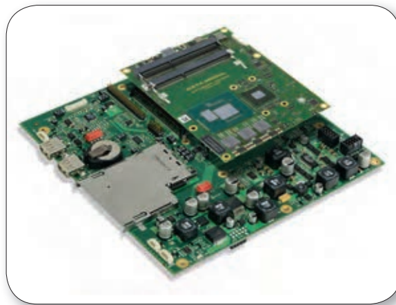
Figure 1. Baseboard and COM Express module developed especially for visual solutions
