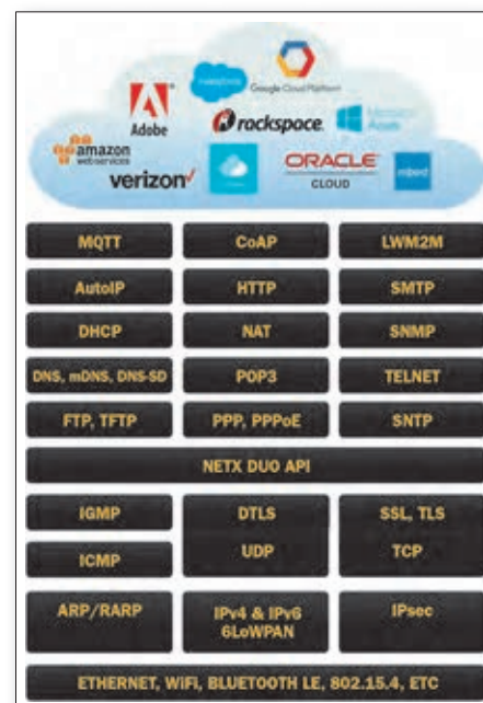
Figure 5. X-Ware IoT Platform is built on top of Express Logic high-performance ThreadX RTOS and NetX Duo dual IPv4/IPv6 TCP/IP stack. The industrial-grade platform adds new IoT protocol support including 6LoWPAN, MQTT, CoAP, and LWM2M for securely connecting the smallest of IoT devices to the cloud.
