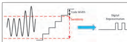
Figure 2. Once the signal crosses the sensitivity level, it is represented by a different digital value.
