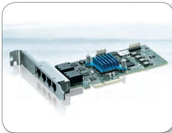
*The standard Kontron network card includes an integrated switch for redundant networks with two or four gigabit Ethernet ports. It meets all specifications of IEEE 802.1 and is especially suited for rough industrial environments.*
