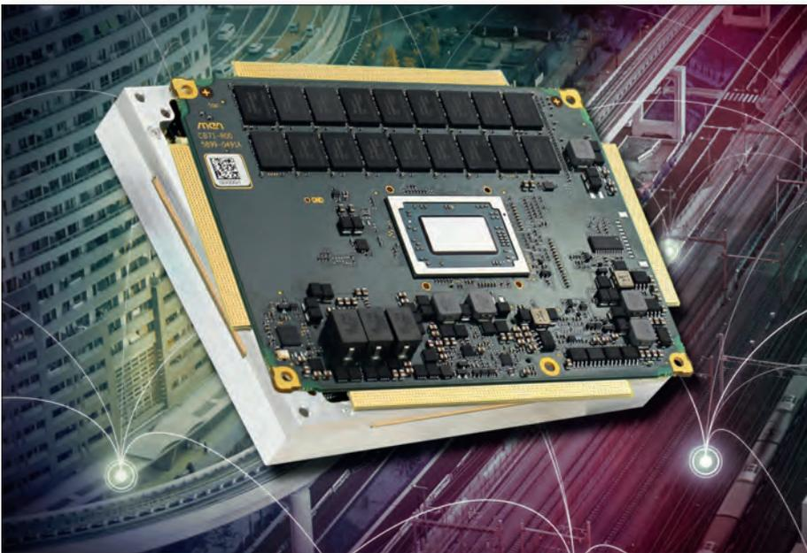
Figure 3. The VITA 59 compliant COM Express Rugged standard allows fanless operation of AMD Ryzen Embedded processors even at TDPs over 35W e.g. on MEN Micro CB71C board.
