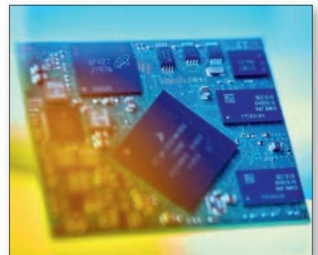
*Figure 1. The TQMa7x mini module, based on the i.MX7 processor from NXP, combines the ARM Dual Cortex-A7 core technology with a variety of interfaces.*
