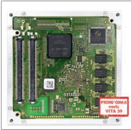
Figure 2. The standard FPGA on the Rugged-COM Express module CC10C with ARM i.MX6 processor provides flexible, customizable I/Os.
