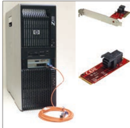
Figure 5. Just by integrating one COTS PCIe or M.2 adaptor to miniSAS-HD card, you can add myOPALE-IO on the front panel of your PC for audio, broadcast, communication extensions.
