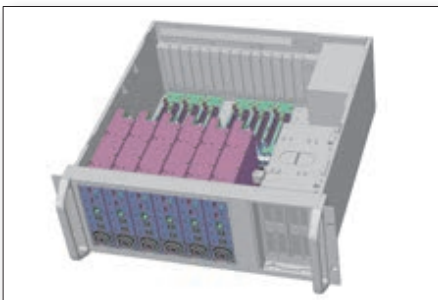
Figure 4. Blade with expansion slots demonstrates the capability to integrate 6-in-1 system in 4U/19" rackmount. Each blade can drive up to two I/O cards.
