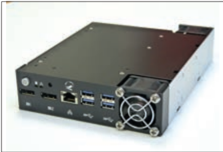
Figure 3. myOPALE-CPU building block in half-height 5.25" form factor with its own monitored cooling system mixing conduction cooled and push-pull airflow technologies.
